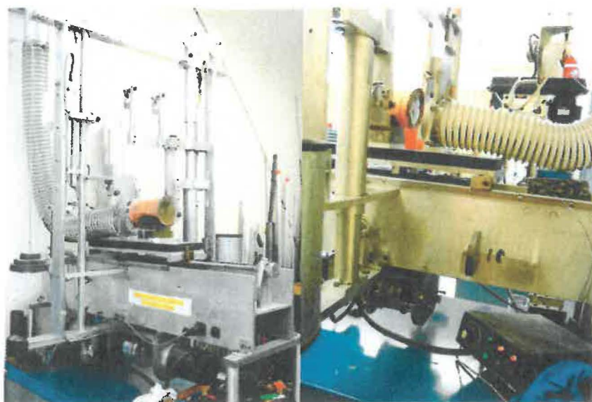
Figure 4. Diamond wire saw with ventilation, pulley system, adjustable table, wheel, pump and pump controller
